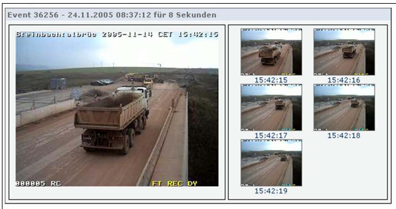
Fig. 3. Photos for securing evidence on the basis of the dynamic recognition of a truck on the joint structure (website)
