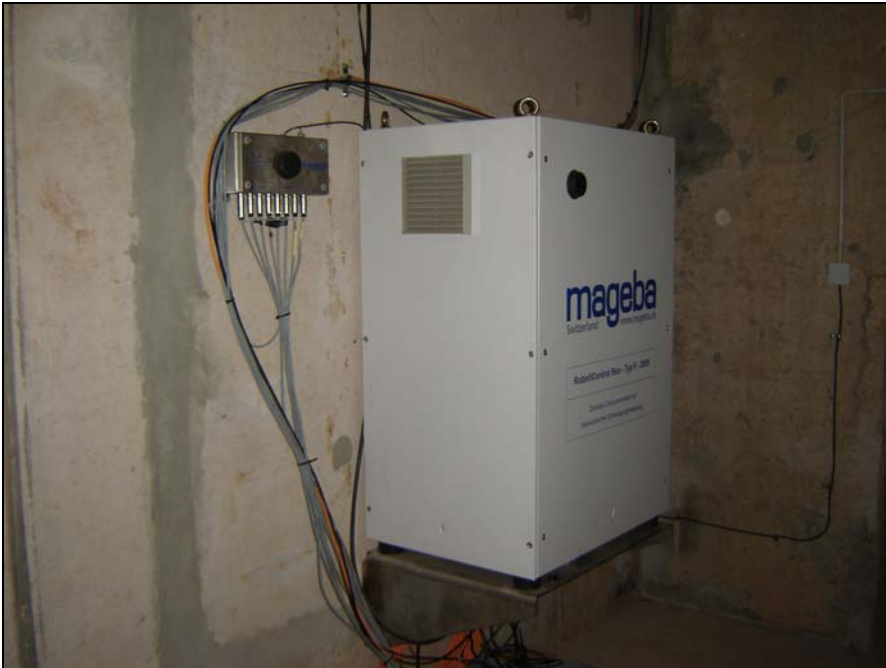
Fig. 4. The measuring data unit, the so called Robo®Control Box of Type I for conventional measuring (RC-Box I: small, silver coloured) and of Type II with an integrated laser interrogator for dynamic measurements (RC Box II: big, white).
